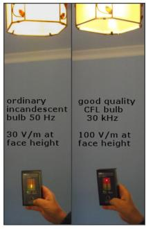
The electric field level often rises towards the ceiling, mainly due to the fields from light fittings and lighting circuit wiring. Some common wiring styles used for lighting circuits produce high fields near the ceiling and light switches.
