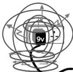
Electric and Magnetic Fields from plug transformer (mains adapter)
